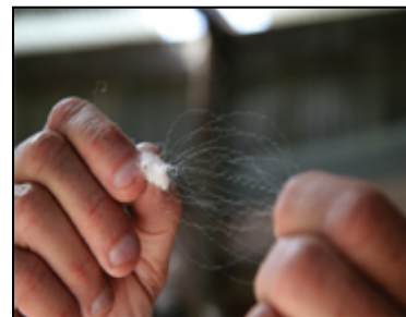
Figure 2. A quick test for fibre uniformity and fibre elasticity.
